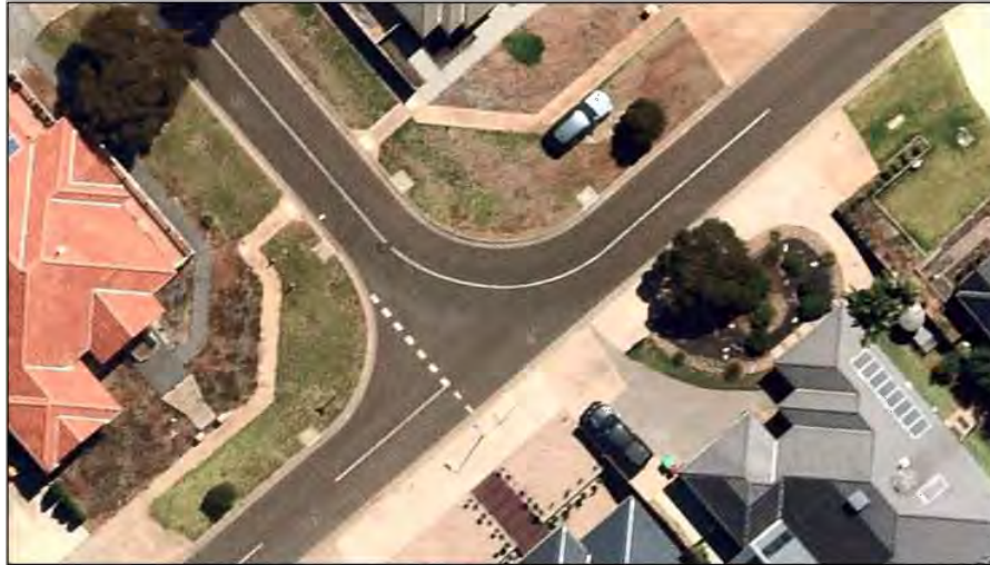
Figure 4 Example of a modified T-intersection (from Nearmap aerial photography)
