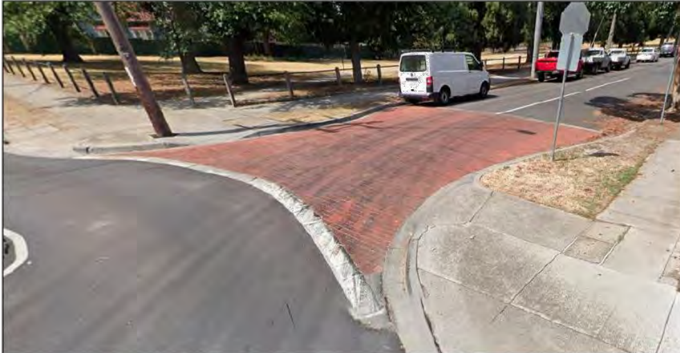
Figure 7 Example of a raised treatment at an intersection (from Google Maps Streetview)
