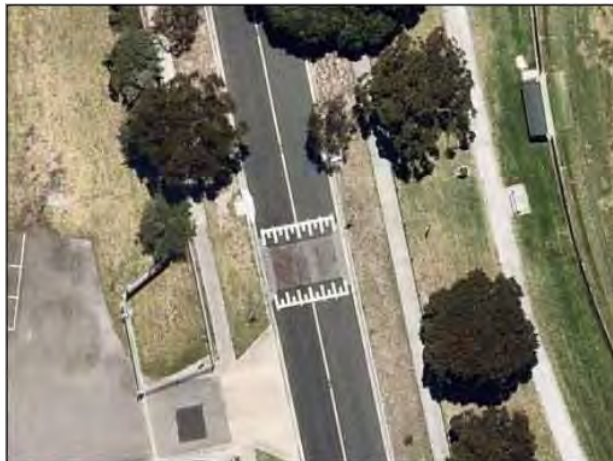
Figure 20 Speed hump on Ti-Tree Crescent to be converted to raised crossing
