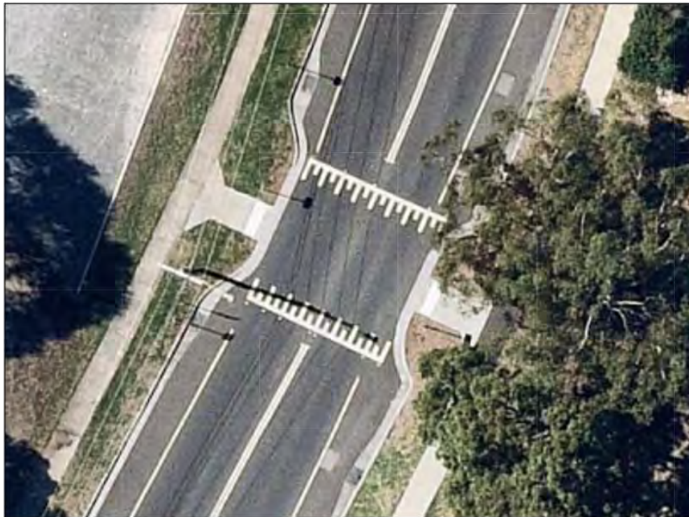
Figure 9 Example of a raised treatment at a pedestrian crossing point, with vehicle priority (Source: NearMap)
