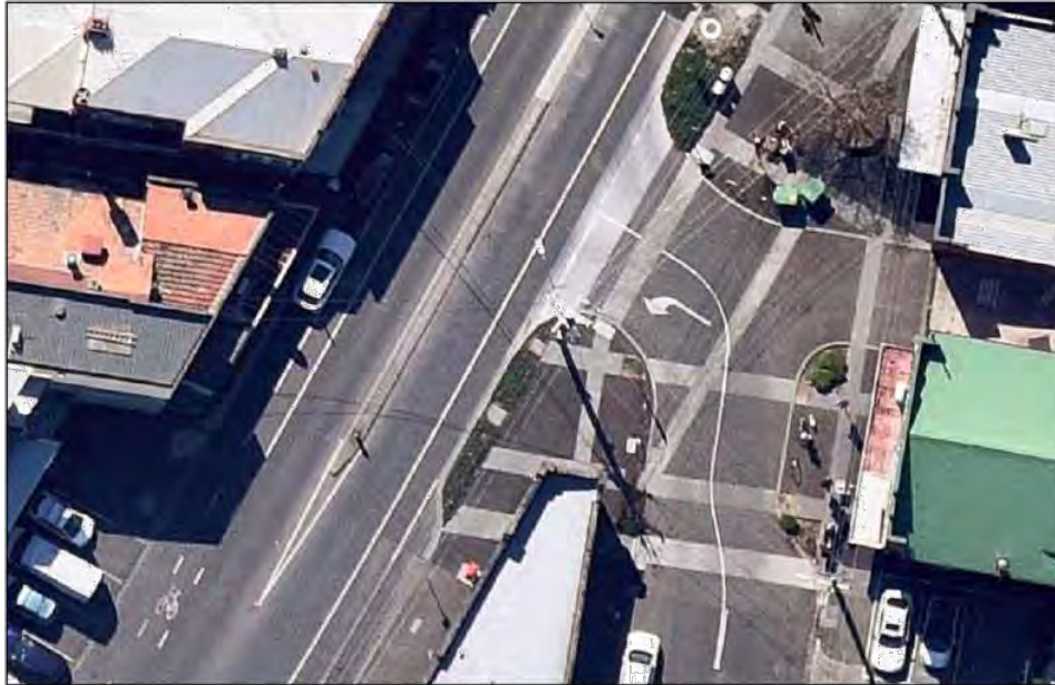
Figure 10 Example of a left-in / left-out treatment (from Nearmap aerial photography)
