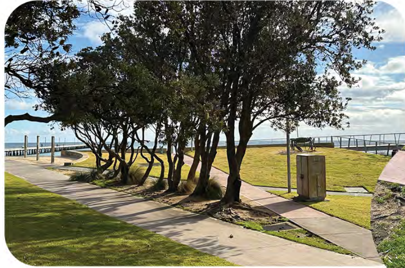
Realign paths away from compacted tree roots (trip hazard, but also long-term risk to tree survival).
