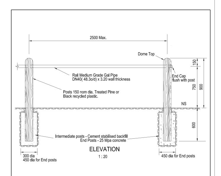
Rail - DN40 Medium Grade (48.3 OD x 3.20 wall thickness) Gal Pipe. Rail in continuous lengths through neat fitting hole in posts with screw & socket splice joins at 6500 intervals. Alternatively butt join (minimum 3 panel lengths) centrally within post with internal sleeve joiner.
