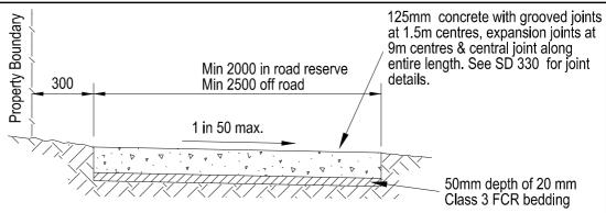
NOTE: Concrete strength min. 25 Mpa at 28 days.
